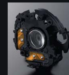
Ceramic ball support system provides compact, high-precision performance
